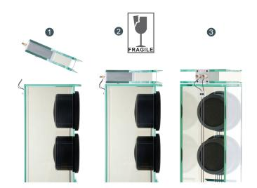
When the speaker is in place then position the glass horn as shown.
