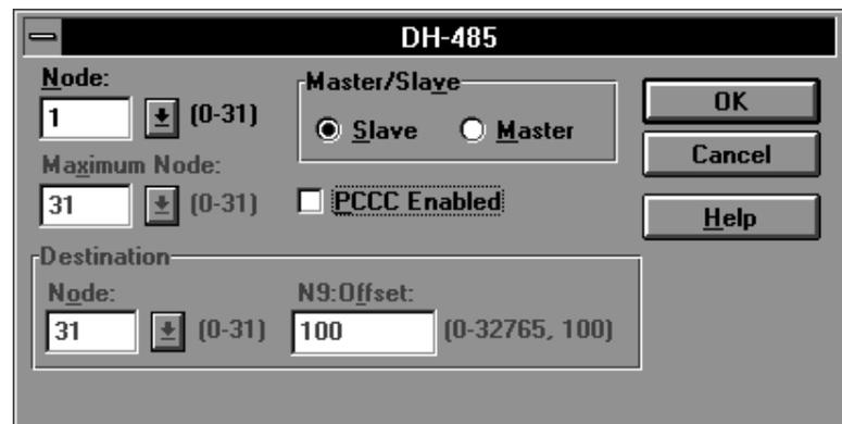
The Message dialogs define the format and content of message data sent to the host by the reader when bar codes are decoded. This dialog is accessed by selecting Message in the Project dialog.
