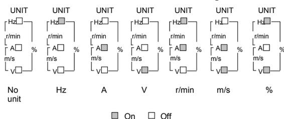
**Fig. 4-3 Unit represented by combination of the indicators**
