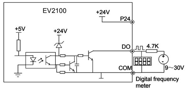
**Fig. 3-31 Wiring 2 of output terminal DO**
