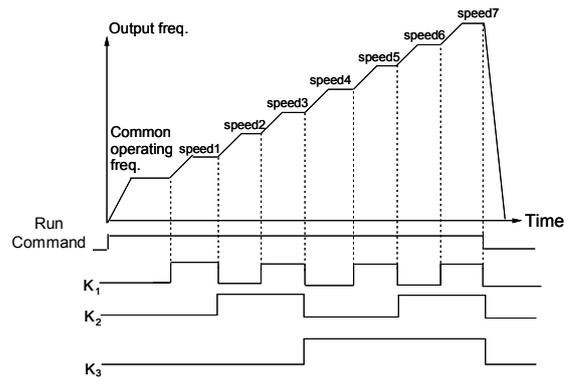
**Fig. 5-194 Multi-step operation**
