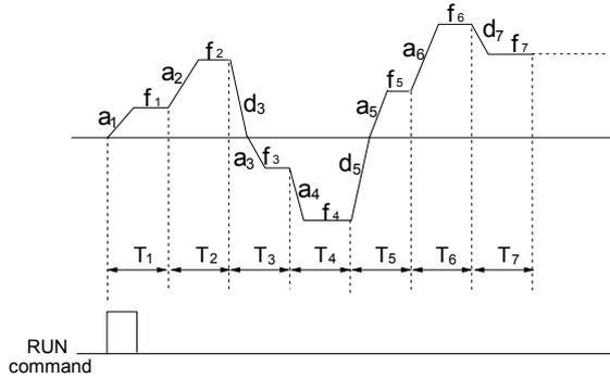
**Fig. 5-22 Maintain the frequency after single cycle**
