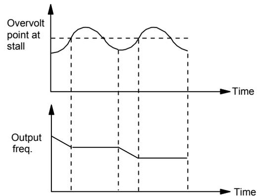
Fig. 5-63 Over-voltage at stall
