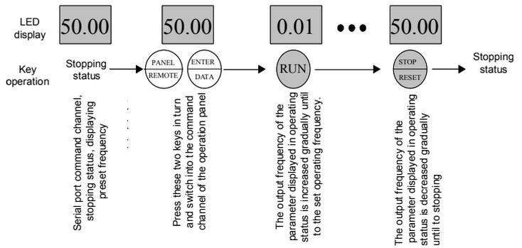
**Fig. 4-11 Operation example for running and stopping**
