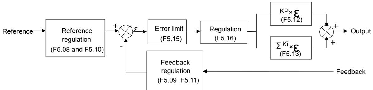
**Fig. 5-28 PI control diagram**
