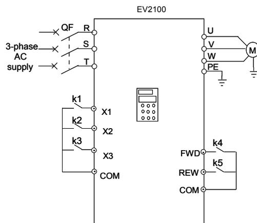
**Fig. 5-35 Wiring for multi-speed operation**
