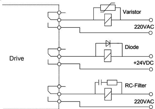
Fig. 3-41 Relay, contactor and electro-magnetic braking kit
