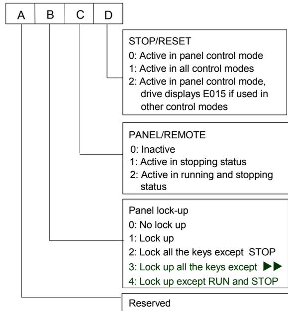
**Fig. 5-58 Functions of keys**
