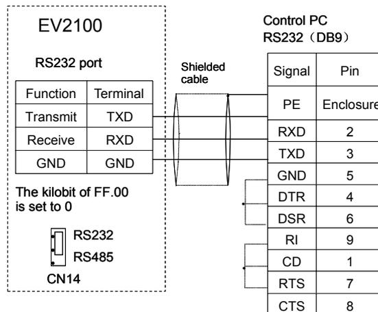
**Fig. 3-17 RS232-RS232 communication cables**
