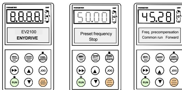
**Fig. 4-4 Displayed during initialization, STOP, operation**
