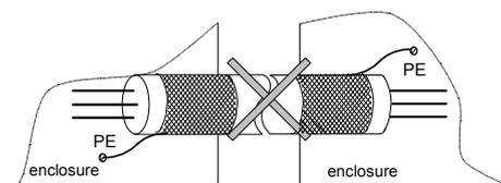
Fig. 3-36 Incorrect earthing method of shielding layer
