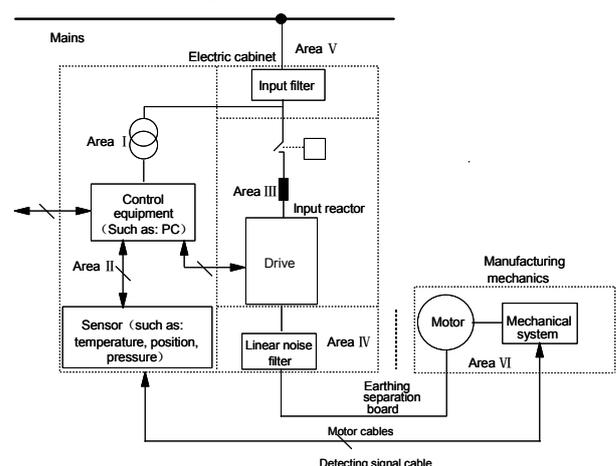
**Fig. 3-43 Recommendation of Installation space**
