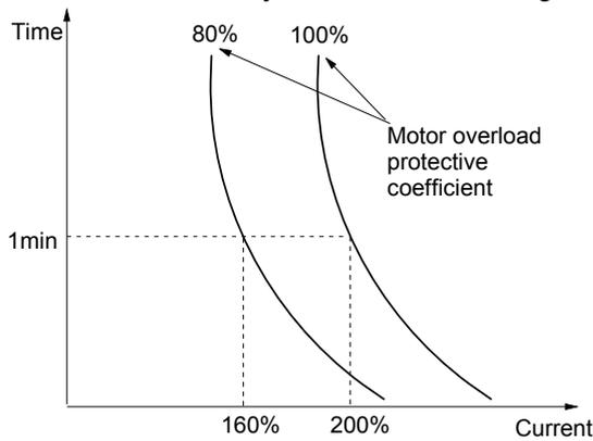
Fig. 5-62 Motor's overload protection coefficient
