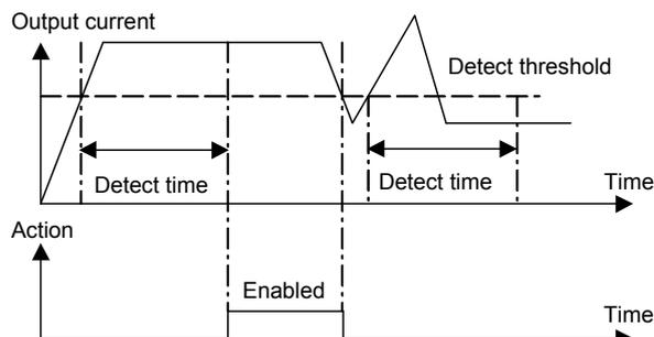
**Fig. 5-65 Overload pre-alarm function**
