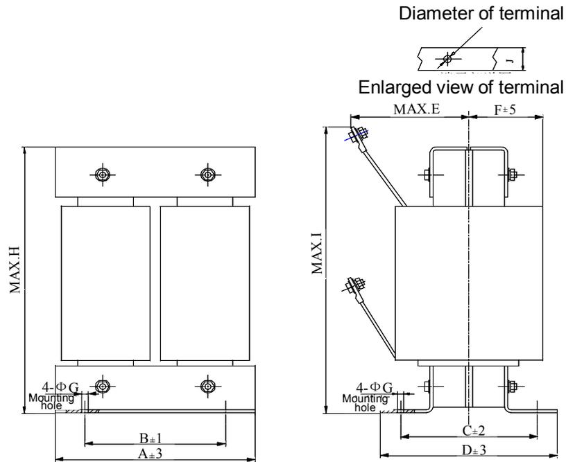
**Fig. 2-3 Dimensions of DC reactor**
