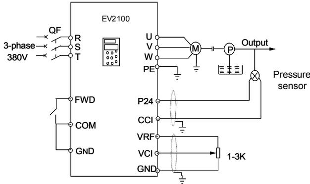
**Fig. 5-27 Analog feedback control system with internal PI**
