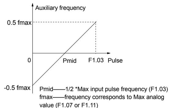
**Fig. 5-56 PULSE-0.5×F1.03 as auxiliary ref. setting method**
