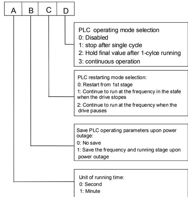
Fig. 5-20 Simple PLC operation mode
