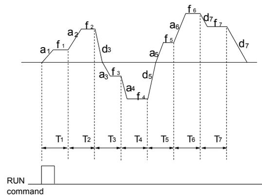
Fig. 5-21 Stop after single cycle of PLC
