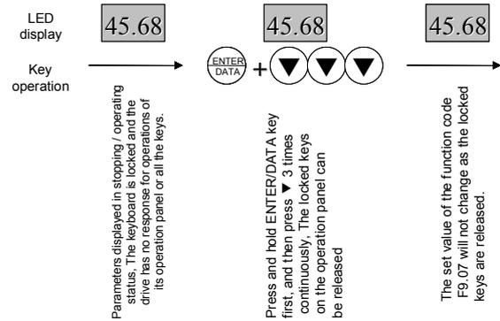
**Fig. 4-15 Operation example for unlocking the operation panel keys**
