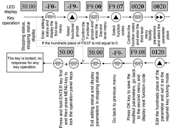
**Fig. 4-14 Operation example for locking the operation panel keys**
