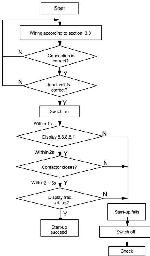
Fig. 4-16 Procedures of first time drive start up
