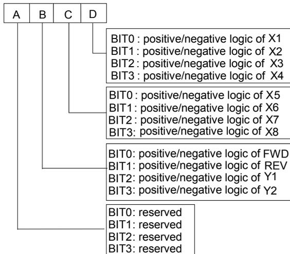
Fig. 5-45 Terminal's positive and negative logic
