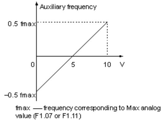
**Fig. 5-55 VCI-5/CCI-5 as auxiliary ref. setting method**
