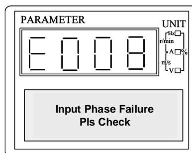
**Fig. 4-5 Parameter displayed in alarm status**
