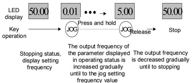
**Fig. 4-12 Operation example for jog running**
