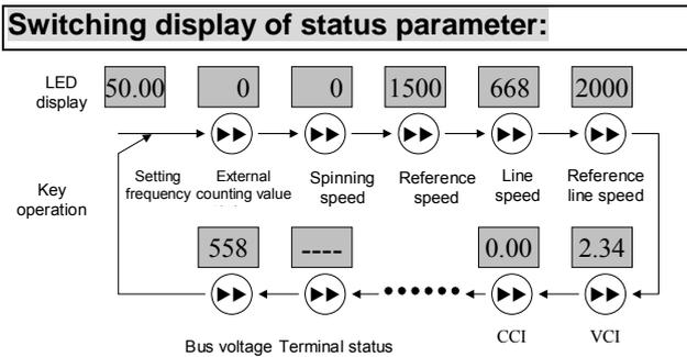
**Fig. 4-7 Operation example for displaying parameters in stopping status**
