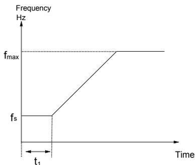
Fig. 5-12 Starting frequency and starting time
