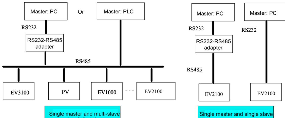
Fig. A-7 Networking diagram of drives
