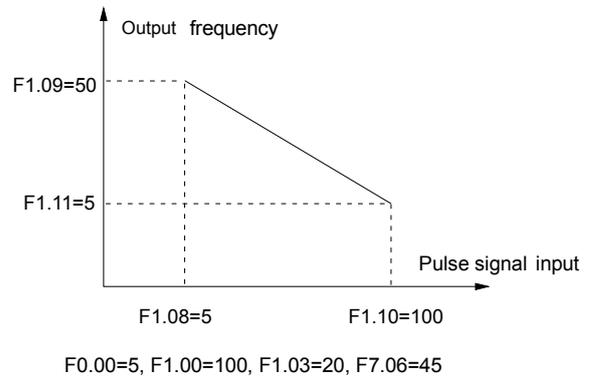
Fig. 5-10 Pulse signal input
