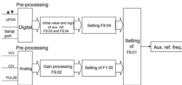
**Fig. 5-54 Auxiliary reference frequency selector**
