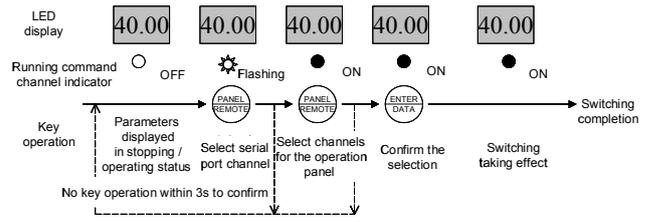
**Fig 4-10 Operation example for switching running command channel**
