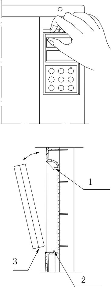
**Fig. 3-4 Removing and Mounting of Operation Panel**
