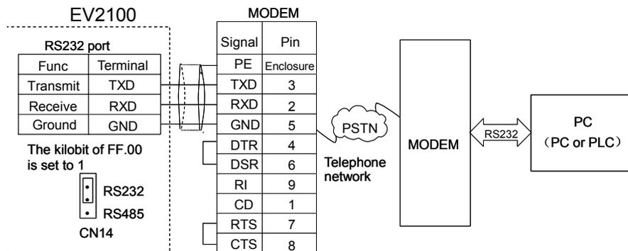
**Fig. 3-19 Wiring of RS232-(MODEM-PSTN-MODEM)-RS232 communication**
