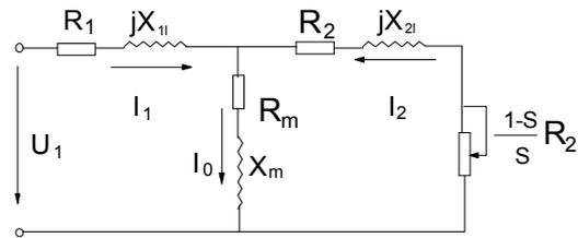
Fig. 5-61 Motor's equivalent circuit
