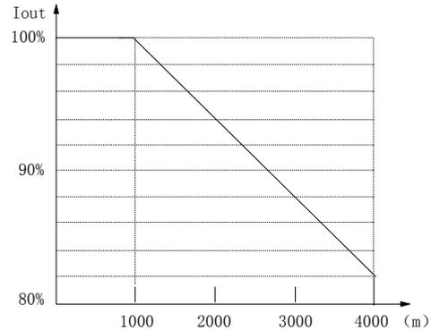
**Fig. 1-3 Derating Drive's output current with altitude**
