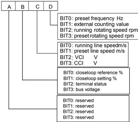
Fig. 5-49 Stopping parameters displayed by LED
