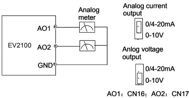
**Fig. 3-16 Wiring analog output terminal**
