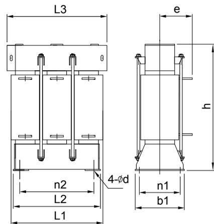
**Fig. A-3 Outline of 3-phase AC input and output reactor (c)**
