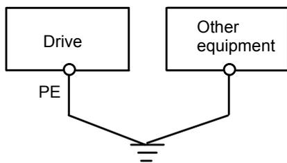
Fig. 3-38 Earthing diagram 2
