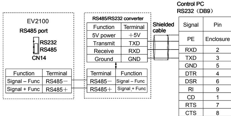
**Fig. 3-18 RS485-(RS485/RS232)-RS232 communication cable**
