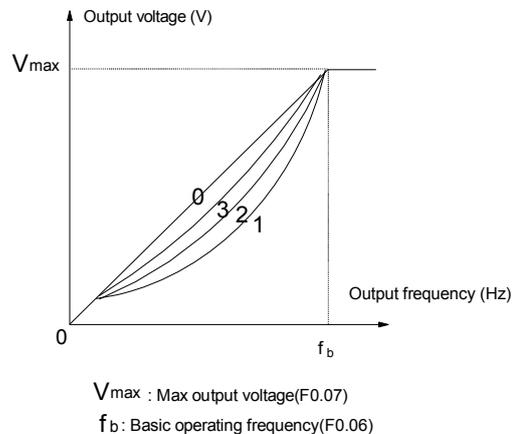
**Fig. 5-5 Torque-reducing curve**
