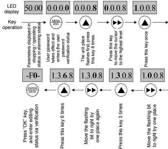
**Fig. 4-13 Operation example for unlocking user password**
