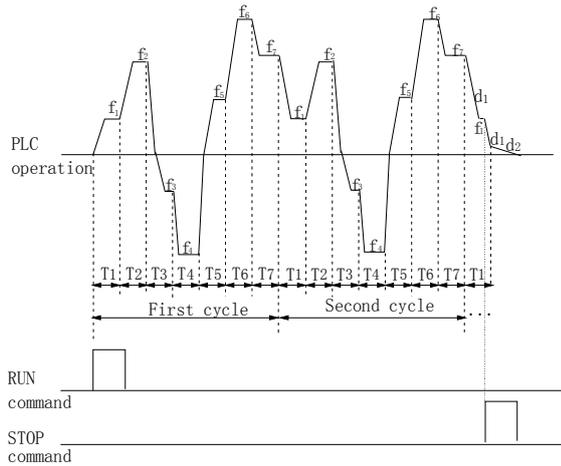
**Fig. 5-23 Continuous operation of PLC**
