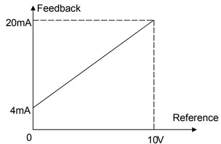
**Fig. 5-29 Reference and feedback**
