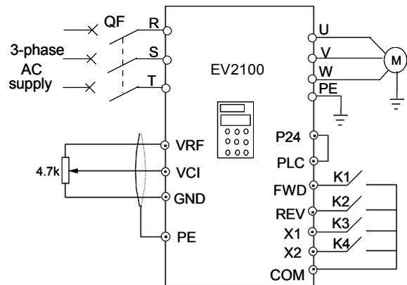
**Fig. 5-52 Remote and local control connection**
