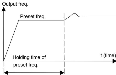
**Fig. 5-33 Preset frequency of close-loop operation**
