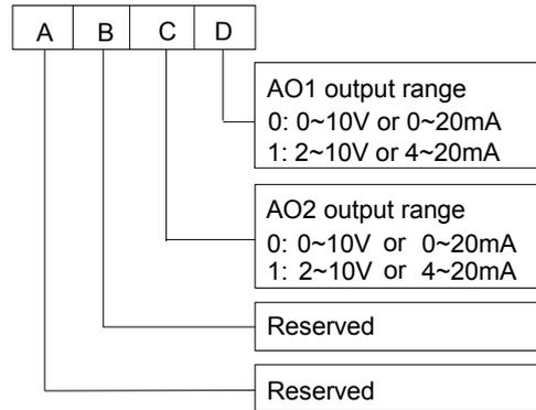
**Fig. 5-43 analog output offset settings**
