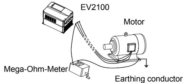
Fig. 1-1 Checking the insulation of motor
