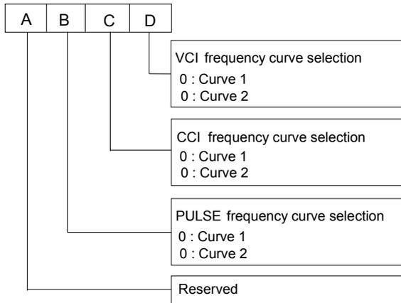
Fig. 5-9 Frequency curve selection
