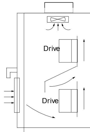
Fig. 3-3 Installation of several drives
