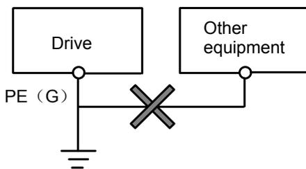
Fig. 3-40 Earthing diagram 4
