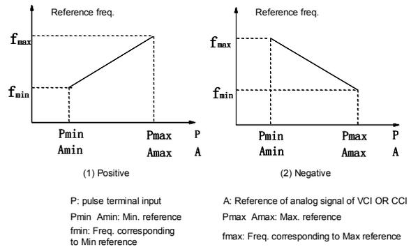
Fig. 5-8 Output frequency characteristic curve
