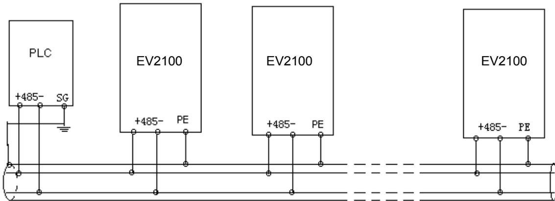
**Fig. 3-21 Communication between PLC and the drive (the drive and motor are grounded well)**
