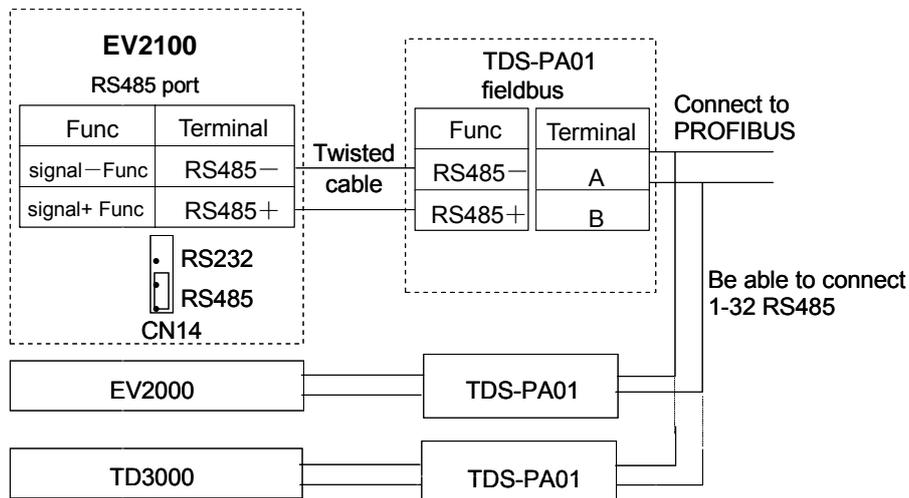
**Fig. 3-20 Wire connections of RS485-(TDS-PA01)-PROFIBUS communication**
