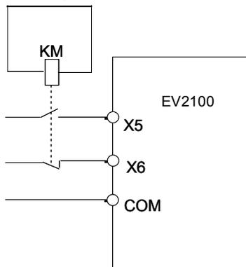
**Fig. 5-36 Normally-open/close input**
