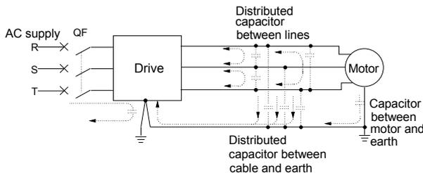
**Fig. 3-42 Flowing path of leakage current**
