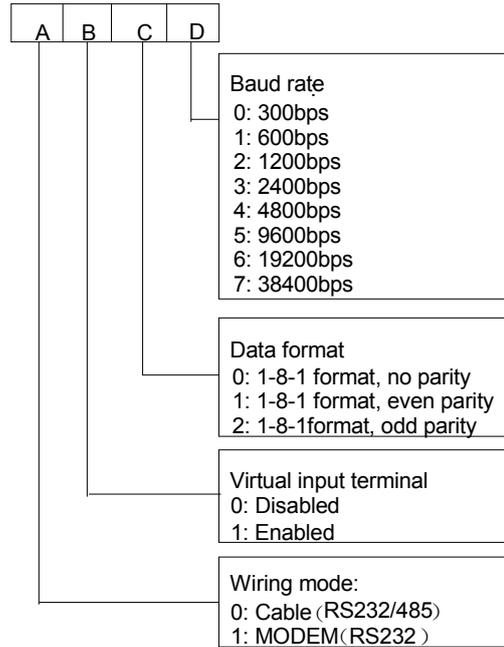
**Fig. 5-60 Communication parameters**
