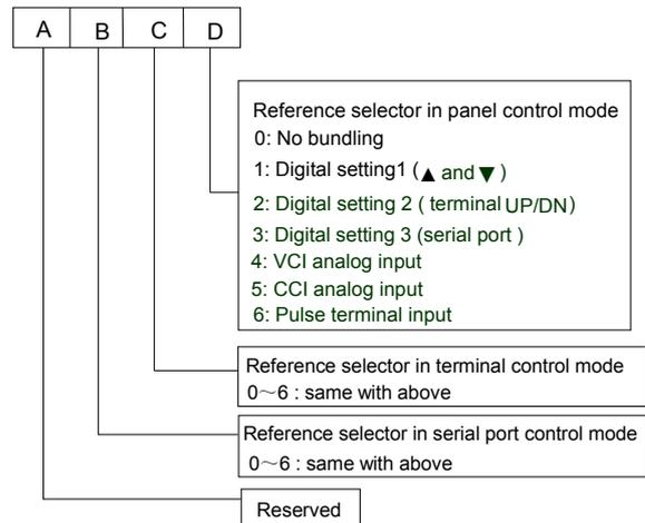
Fig. 5-210 Control mode is bundled to frequency selector
