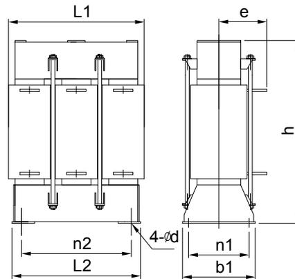
**Fig. A-2 Outline of 3-phase AC input and output reactor (b)**
