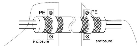
Fig. 3-35 Correct shielding method of shielding layer
