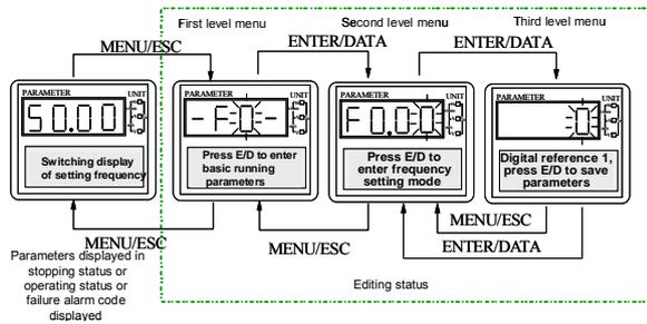
**Fig. 4-6 Programming display status of the operation panel**
