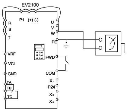
**Fig. 7-1 Insulation test of drive**
