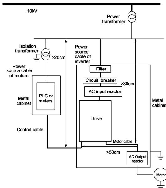
**Fig. 3-44 Installation of the drive**
