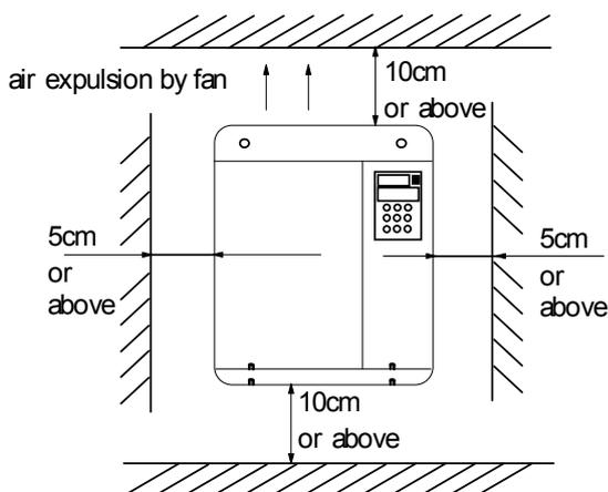
Fig. 3-1 Installation clearance (55kW or below)
