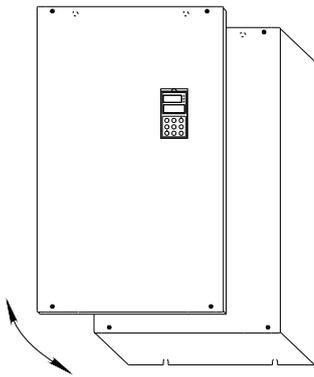
**Fig. 3-6 Removing and mounting metal cover**
