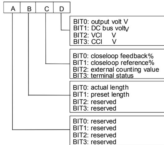
**Fig. 5-47 Operating parameter 2 displayed by LED**
