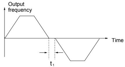
**Fig. 5-15 Hold time of zero frequency**
