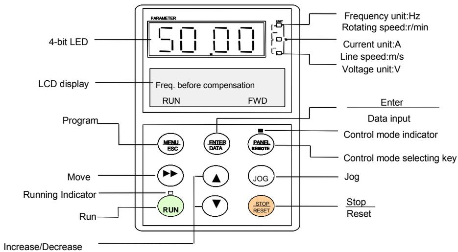
Fig. 4-2 Illustration of operation panel
