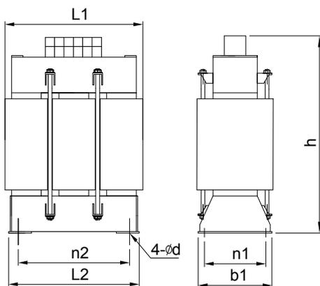
**Fig. A-1 Outline of 3-phase AC input and output reactor (a)**
