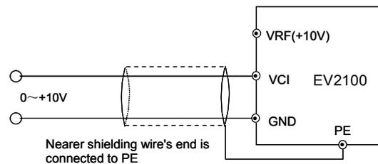
**Fig. 3-14 Wiring terminal VCI**
