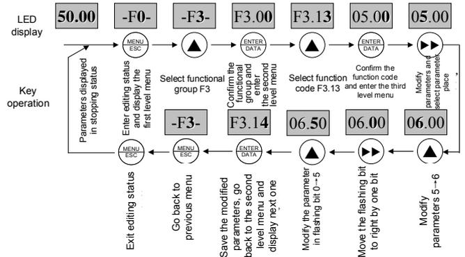
**Fig.4-8 Operation example of editing parameters**
