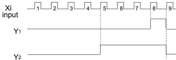
Fig. 5-44 Preset and specified pulse number
