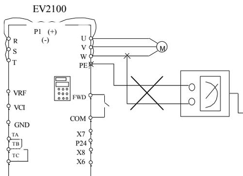
**Fig. 7-2 Insulation test of motor**
