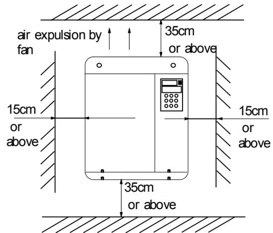
Fig. 3-2 Installation clearance (75kW or above)
