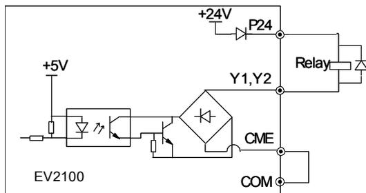
**Fig. 3-28 Wire connections 1 of multi-function output terminal**
