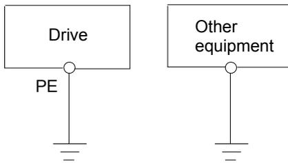
Fig. 3-37 Earthing diagram 1
