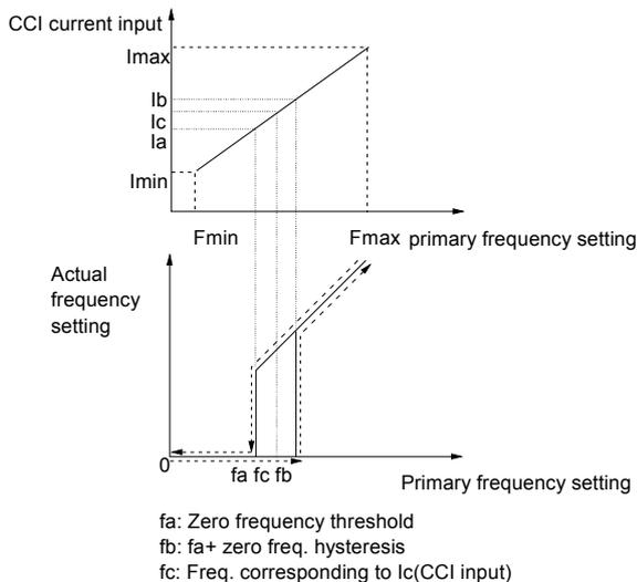
**Fig. 5-59 Hysteresis of zero-frequency operation**
