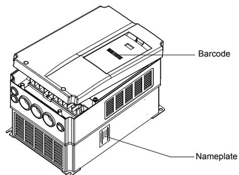
**Fig. A-2 Locations of Nameplate and Barcode**
