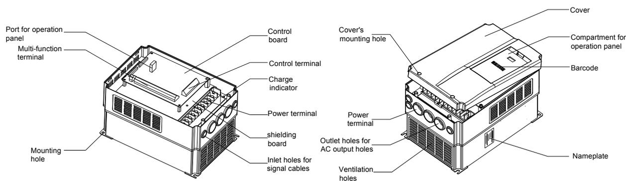
**Fig. 2-1 Structure of drive**
