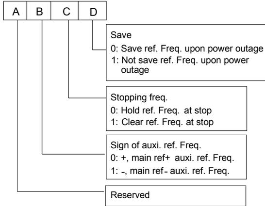
**Fig. 5-57 Digital auxiliary reference frequency control**
