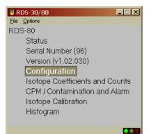
The Configuration Software (CSW) is used to check the status of the instrument, to change its operational parameters and to set-up the histogram operation (for details see the CSW Configuration Software for RDS-80A User's Manual)
