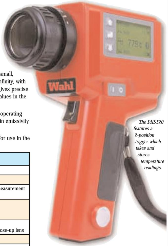
The DHS520 features a 2-position trigger which takes and stores temperature readings.
