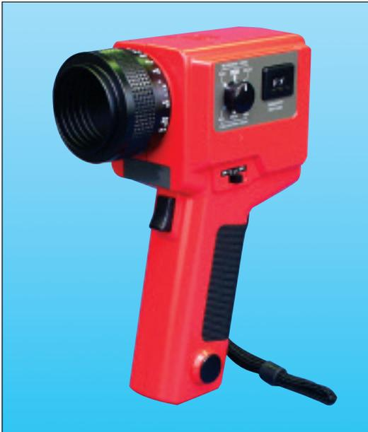
DHS55 – For Liquid Metals - is designed for accurate temperature measurement of liquid metals in iron and steel foundries. The thermometer automatically compensates for ambient temperature changes, and provides a fast response time (0.8 seconds) and reliable reading in the extended range of 1830° to 3270°F (1000° to 1800°C). Short wavelength operation (0.55µm) minimizes errors due to emissivity/atmospheric absorption.
