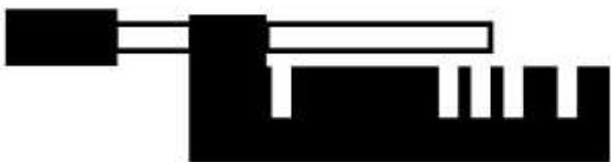
Cross-Section of Shoulder Align Key Fixed
