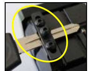
3. Put the bolt into middle hole of the auxiliary key clamp set and fasten it to press the key.
