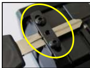
2. Place the auxiliary key clamp set on the clamp and loosely fasten the bolt.
