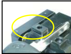
2. Insert the auxiliary key clamp set into the deeper groove between the two sides of the key.
