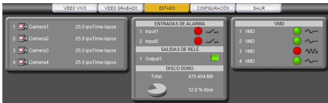
Fig. 41 – VX4BOX/VX8BOX status screen
