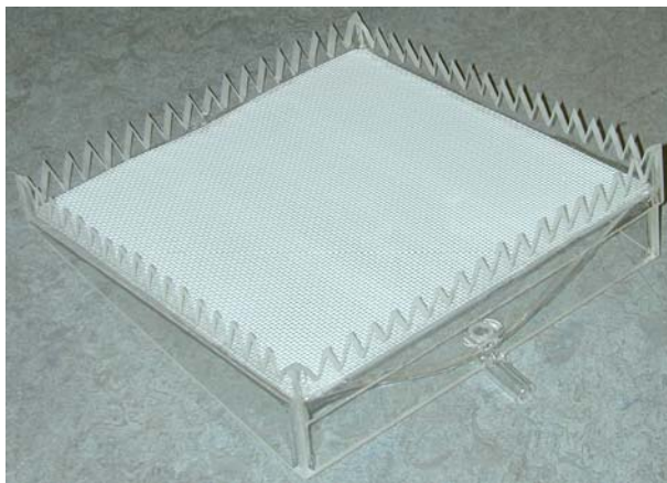
Figure 10. Percolation lysimeter (Note that the lysimeter drains freely through a tube connected to a 5-L collection container (poly-propylene), which is graded to allow the field recording of the collected volume.
