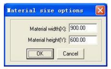
**Material width(X):** It is the width of the work piece (the default is the worktable's width).
