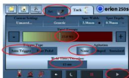
1. Use the provided stylus to select 25Ws energy, max time on the weld time bar, no agitation, trigger on touch, then hit play.
