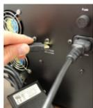
3. Plug the foot pedal into any of the three "Foot Pedal/Microscope" ports on the welder. Use of foot pedal is optional.
