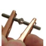
4. Plug the Alligator clips into the Tack ports then line up the work pieces and step on the foot pedal.
