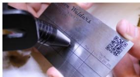
2. Lightly touch the electrode in the 25Ws box on the provided weld plate. Maintain contact & keep hands steady by resting them on the table.
