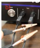
4. Choose your preferred hand piece attachments and plug them into the front of the welder. **\*a) Arc Welding. b) Tack Welding.**
