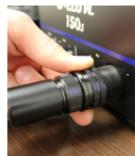
1. With the slit on the Stylus plug facing up, lightly push the plug into the port and screw the connector on the plug clockwise 3 or 4 turns.
