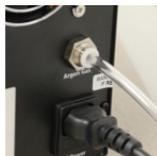
2. Attach the thicker end of tubing to the regulator, then the thinner end to the back of the welder.
