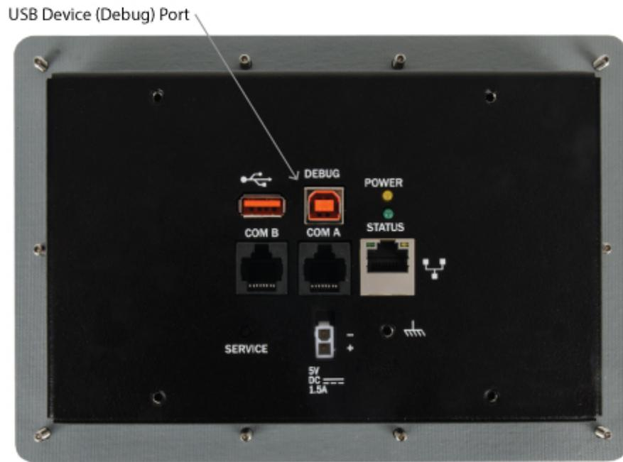
**Figure 30.** Type B USB Connector
