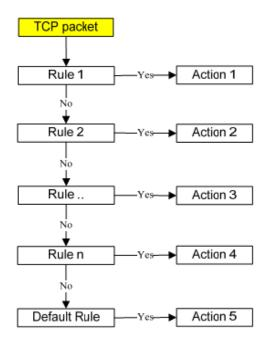
Above: A chain-rule diagram of IP filtering procedures.
