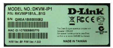
Left: The label on the bottom of each DKVM-IP1 shows the unique MAC ID of the device. This ID is the same as the MAC Address.
