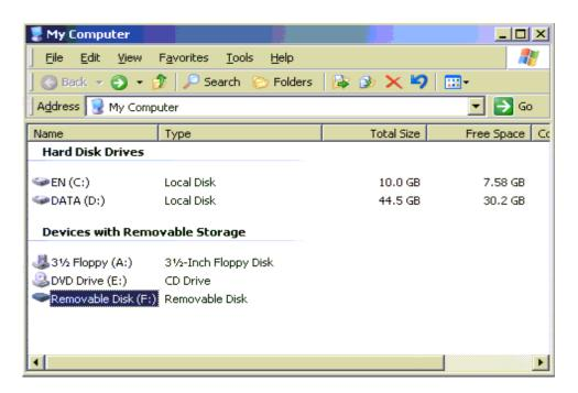
Above: Before using any Virtual Media functions, the Host system should be linked via USB cable to the "USB DATA" port of the DKVM-IP1. After that, clicking on the "My Computer" file view of the Host system should display the DKVM-IP1 as a "Removable Disk".
