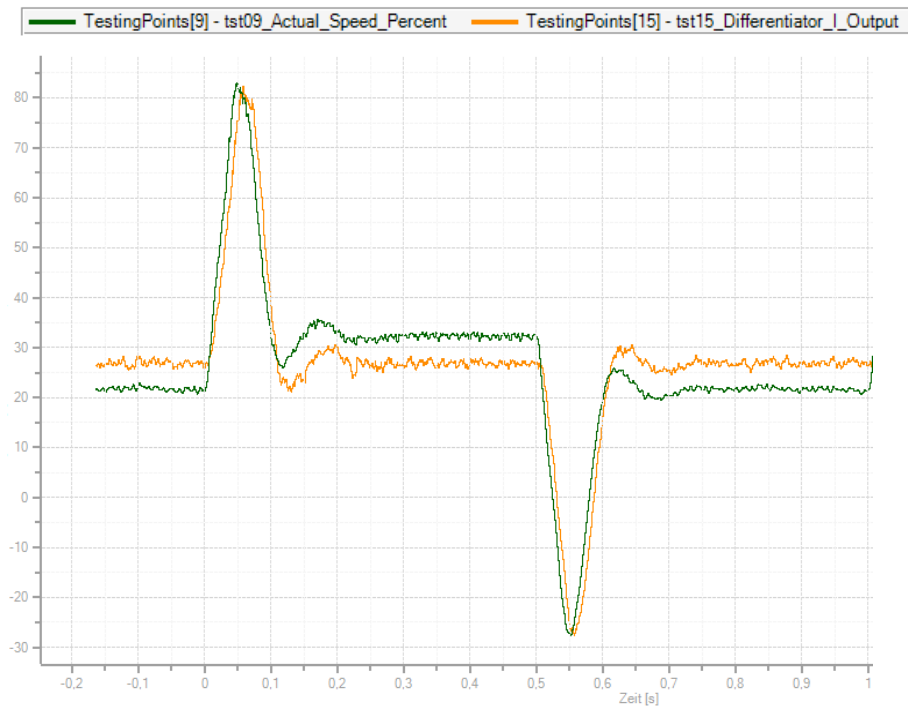
Fig. 4.5 Example behavior without observer ( Derivative_Observer_Gain =0) A phase lag between the two signals is visible.
