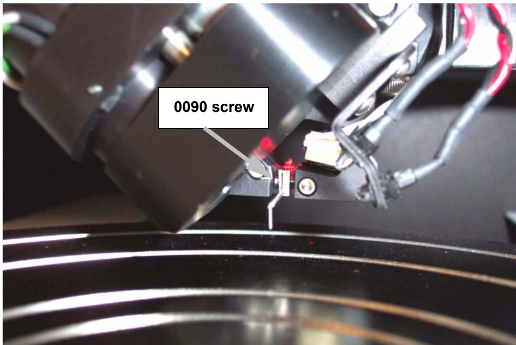
Figure 9.3: The 0090 screw which holds the stylus plate against the shank of the stylus.
