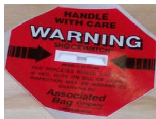
Figure 2.1: Shockwatch™ Monitor used on shipping crate.
