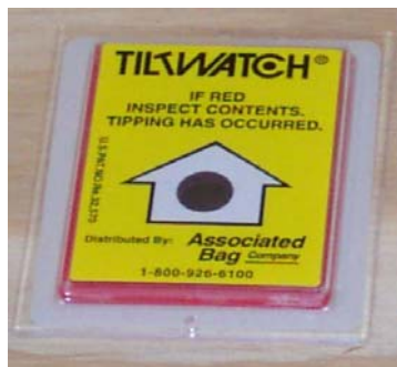
Figure 2.2: Tiltwatch™ Monitor used on shipping crate.
