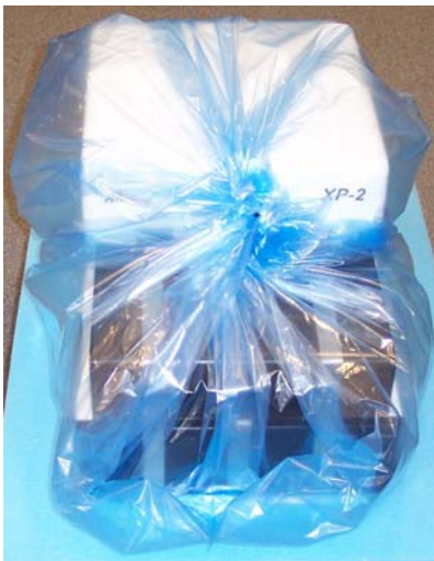
Figure 2.3: XP-2 system wrapped in a plastic bag to keep it clean prior to cleanroom installation.
