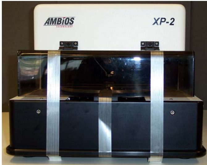
Figure 2.9: Fiberglass threaded tape holding the stage cover closed over the block and stage restraints coming out from under the stage cover door.
