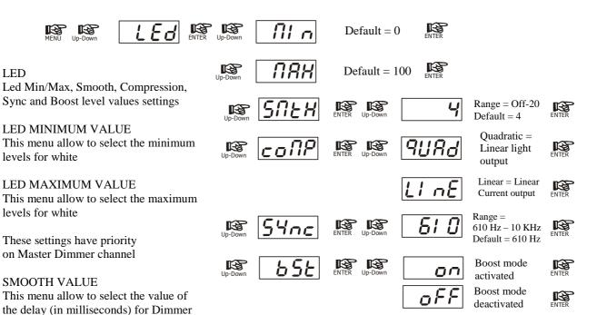
With BOOST active, the LED'S current is set to Max value. (30% more gain compared to **BOOST Off**) Default = Enabled
