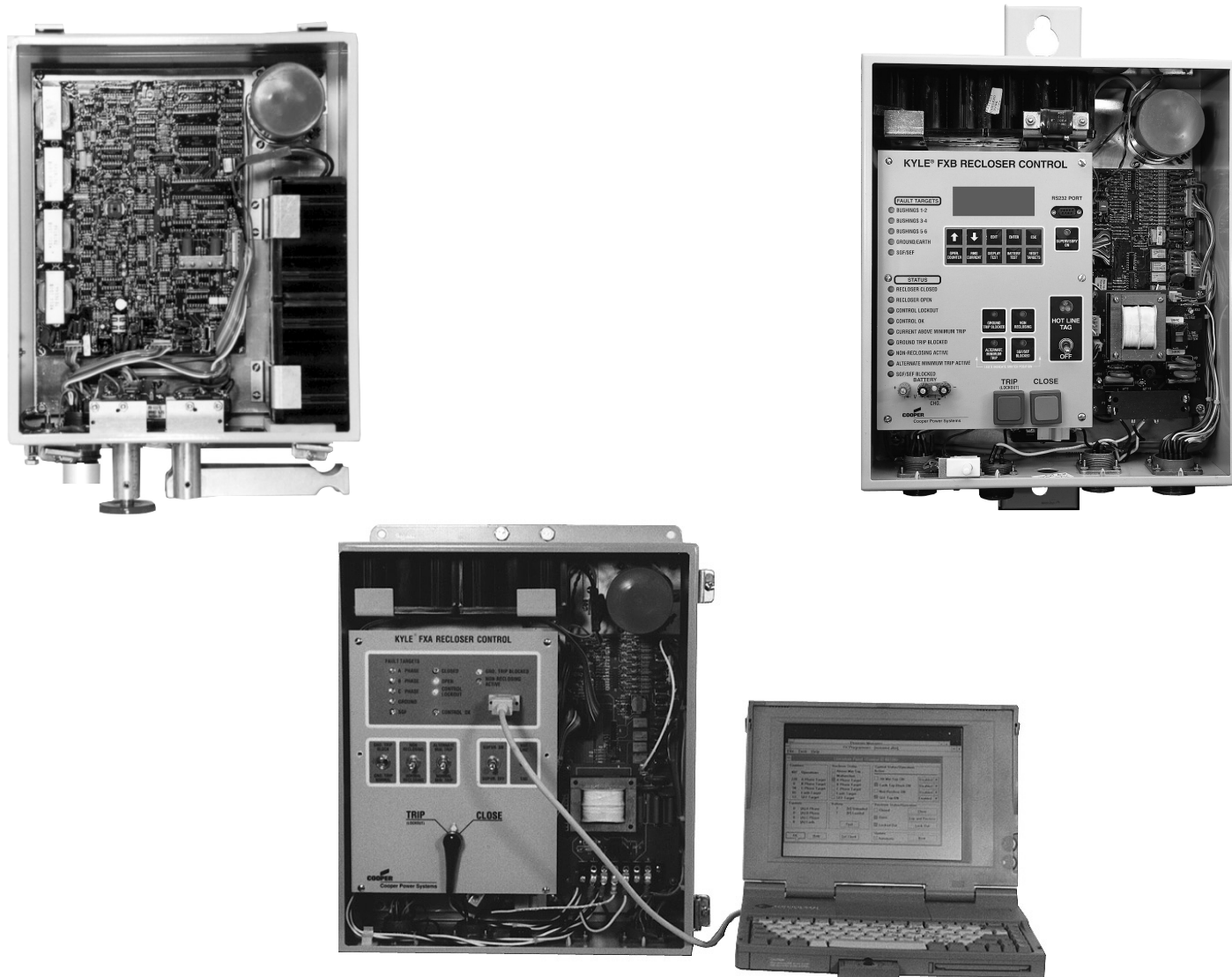
Kyle® Type FX (top left), Type FXA with laptop computer and cable (above; computer and cable not included), and Type FXB (top right) microprocessor-based recloser controls.
