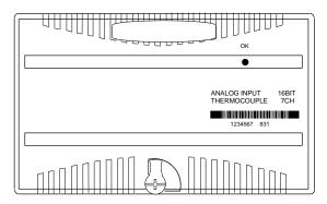
Each input channel can be configured to report millivolts ranges as 1/100 of millivolts, or thermocouple inputs as linearized temperature in tenths of degrees Celsius or Fahrenheit, with or without cold junction compensation.
