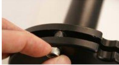
5. Attach the sonar to the sonar clamp by loosening the four cap screws, sliding in the sonar and retightening the four cap screws.
