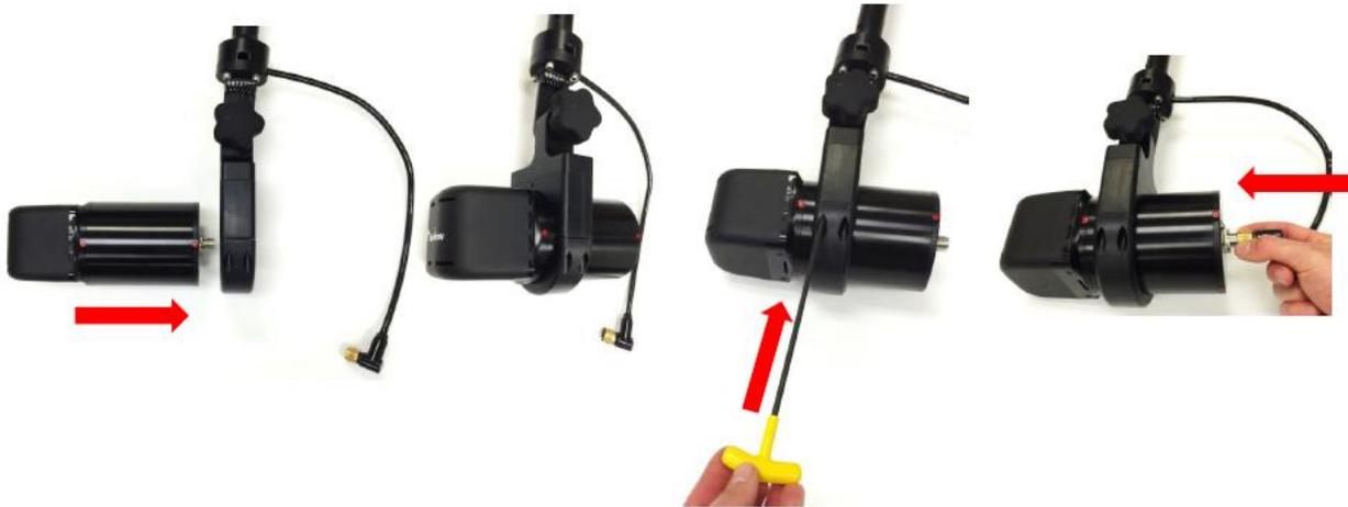
**NOTE:** Use the stickers and connector placement on the rear end cap of the sonar or the logo on the front end of the sonar to determine the up-down orientation of the sonar. If the sonar is inverted, be sure to select the “inverted” option in ProViewer’s settings.
