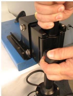
3. Rotate the pole in the mount so that the sonar, when set to the 'home position,' points in the desired direction.
