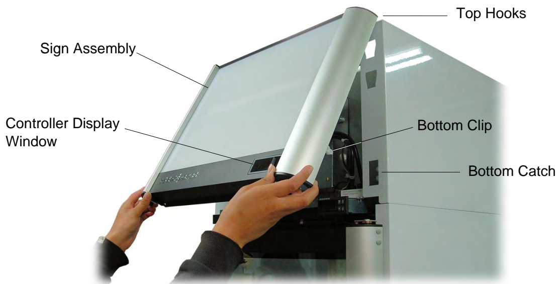
Figure 6: Fitting the Sign Assembly
