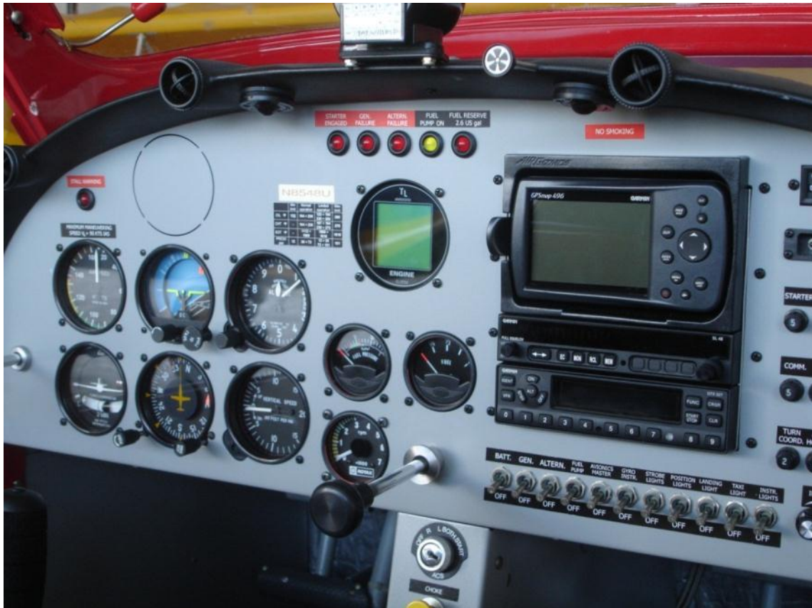
Figure 3-2. Gauges to be implemented. The “Six-pack” gauges are the cluster of six large gauges to the left of the picture. Photo by Robert Gysi.
