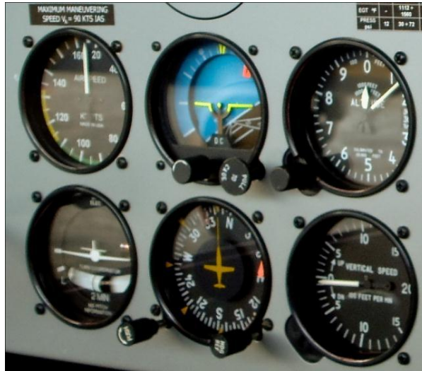
Figure 2-11: This is the standard six-pack of gauges in the GoBosh. Photo by Robert Gysi.
