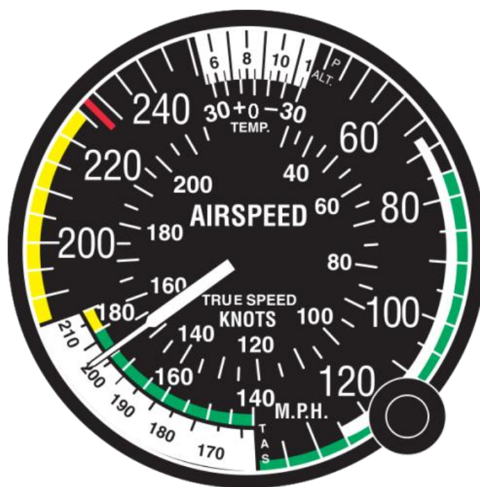
Figure 3-20. Airspeed Indicator Faceplate - Wikipedia. Used with permission under the GNU Free Documentation License 9
