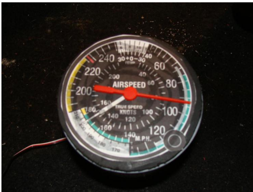
Figure 3-42. Assembled flight instrument with face plate and needle. Photo by Joseph Munera
