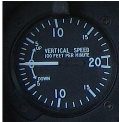
Figure 3-23. Face plate of the vertical speed indicator. This work has been released into the public domain by the copyright holder, Benet Allen. 11
