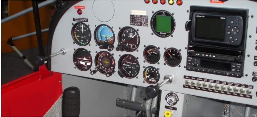
Figure 3-50. Throttle location (black knob pulled out of instrument panel). Photo by Robert Gysi
