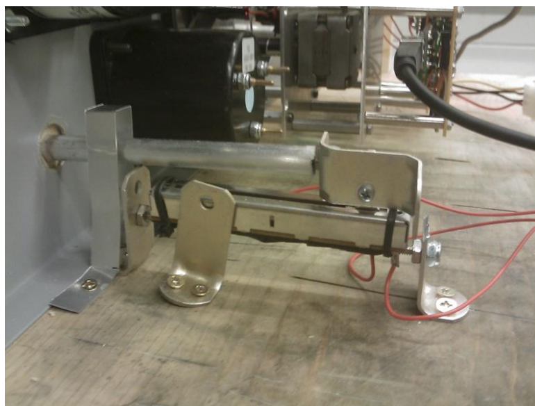
Figure 3-54. Completed throttle assembly. Photo by Robert Gysi
