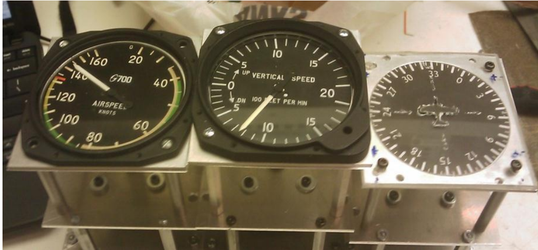
Figure 3-39. Assembled face plates for a various flight instruments. Photo used with permission from Lewis Vail
