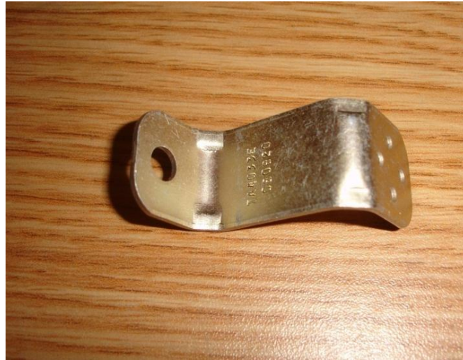
Figure 3-53. Angle bracket for connecting to slide potentiometer. Photo by Robert Gysi
