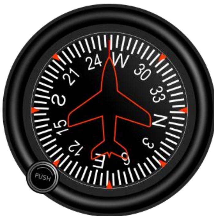
Figure 3-33. Face plate of the heading indicator. Used with permission under the GNU Free Documentation License 19
