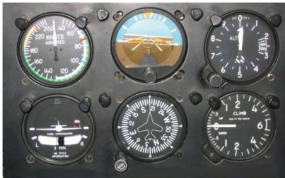
Figure 3-11. Closeup of the standard “Six-Pack” – Wikipedia used with permission under the GNU License 6
