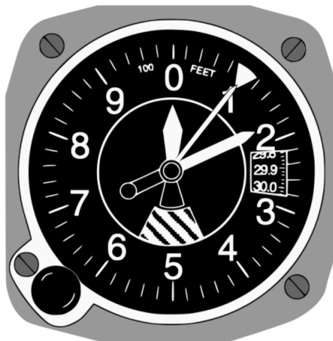
Figure 3-17. Altimeter Face plate, dials, and barometric pressure adjustment knob. This image has been released into the public domain by its author, Bsayusd at the Wikipedia project. 7
