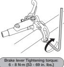
When installing the components to carbon frame/handle bar surfaces, verify with the manufacturer of the carbon frame/parts for their recommendation on tightening torque in order to prevent over tightening that can cause damage to the carbon material and/or under tightening that can cause lack of fixing strength for the components.
