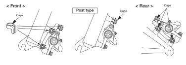
For C-shaped guides and the usual < C-shaped guide > < Usual type of cable stopper type of cable stoppers, use the special Shimano cable supporter (sold separately) to secure as shown in the illustration Tightening torque: 0.3 - 0.5 N·m {2.7 - 4.4 in. lbs.}
