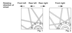
Installation of the rotor SM-RT81L / RT67L (203mm) SM-RT81M / RT67M (180mm) SM-RT81S / RT67S (160mm)
