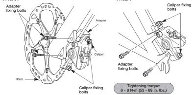
Tightening torque: 6 - 8 N·m {53 - 69 in. lbs.}
