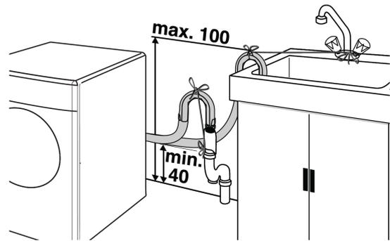
To prevent flowing of dirty water back into the machine and to allow for easy discharge, do not immerse the hose end into dirty water and do not insert it more than 15 cm into the drain. If it is too long, carefully cut it shorter.
