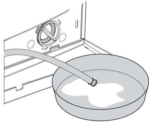
a. Pull the emergency draining hose out from its seat
