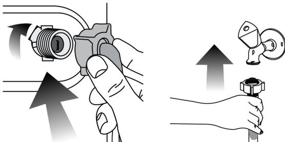
3. Open the taps completely after finishing the hose connection and check for water leaks. If there are any leaks, turn off the tap and remove the nut. Retighten the nut carefully after checking the seal. To prevent water leakages and damages caused by them, keep the taps closed when the machine is not in use.
