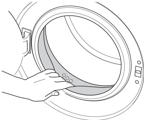
If the holes on the bellow (shown in the figure) are blocked, carefully open the holes using a toothpick.
