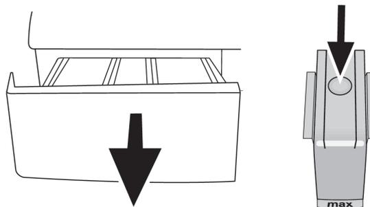
1. Press the dotted point on the siphon in the softener compartment and pull it towards yourself until the compartment is removed from the machine.
