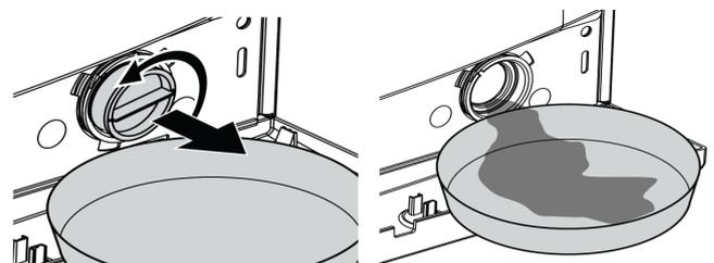
a. Place a large container in front of the filter to catch water from the filter.
