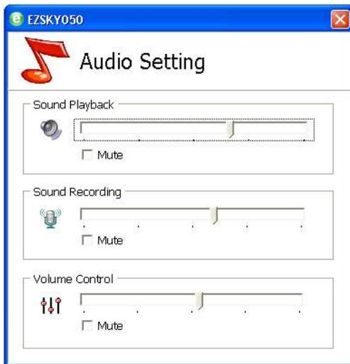
Sound Playback : To setup the volume of the horn
