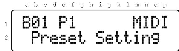
To switch/toggle the Global Setting and Preset Setting, press the **DEC↓(DOWN)** or **INC↑(UP)** switch. And press **ENTER(EDIT/2ND)** switch.
