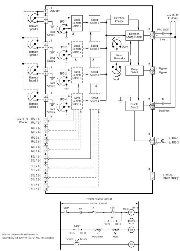
Figure 7.3 Linear Accel/Decel Control Module Wiring
