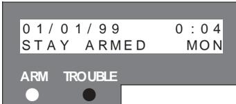
8. Any STAY zones (shown by a steadily illuminated indicator) will be automatically bypassed.
