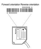
Normally, the unit can read bar codes regardless of the orientation.
