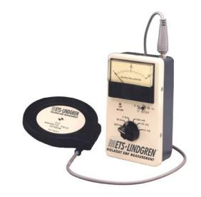
The HI-3624A is a single axis flux density meter designed to be responsive to either sinusoidal or complex magnetic fields. It directly displays the root-mean-square (rms) value of magnetic flux density on an analog meter. The sensor consists of a multi-turn loop connected to the instrumentation readout package via a one meter long cable.
