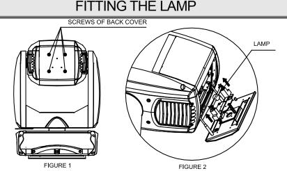
Lock the yoke before fitting/replacing the lamp.
