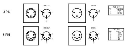
Connection between controller and projector and between one projector and another must be made with a 2 core-screened cable, with each core having at least a 0.5mm diameter. Connection to and from the projector is via cannon 3 pin (which are included with the projector) or 5 pin XLR plugs and sockets. The XLR's are connected as shown in the figure above.
