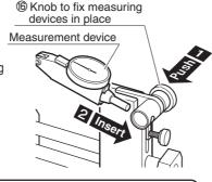
For devices without a carrier, use a holder such as a magnet-base to hold the measuring device in place.
