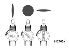
2. Verify trigger slide is in **SPRAY** position (E) and not **NEEDLE REMOVAL** position (D).
