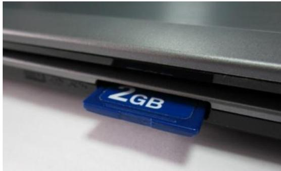
Hold the SD/MMC/MS card with its orientation symbol pointing into the slot and the topside of the card facing up.
