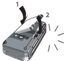
4. Replace the back cover by sliding it until it stops. Remove the protective film covering the screen before using the phone.
