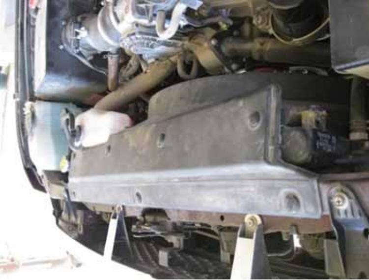
Also take the shroud off, by 5 10mm bolts ( 3 on the overflow bottle, 2 on the radiator shroud.) The shroud is held in th
