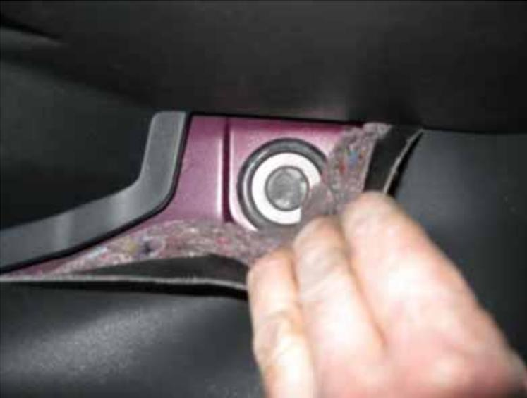
The last one is accessible from behind the cargo area trim. Remove your jack/tools cover and you will see the grommet passenger side is as easy as removing the inverter trim and it is behind that.
