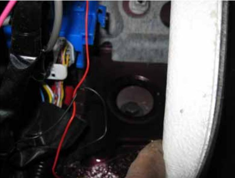
The 3rd one is next to the rear seat. Fold the base of the seat up against the front seats, and from where the child rest floor covering out from under the plastic side trim. The grommet and bolt hole will be exposed in the corner of the floor.
