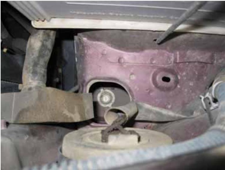
The second is inside the vehicle, close to the firewall. Remove the door sills, foot rest (drivers side) plastic nut and the floor covering up and you will expose a rubber grommet about 2in diameter. pul it out and it will expose the top of the b
