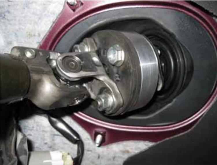
Tighten it good and then proceed to the steering slip joint at the firewall which you loosened earlier and tighten it back
