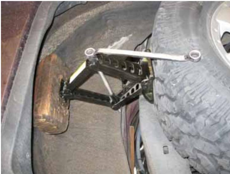
Each wheel you lift from gives you access to 2 body mounts eg. Front Drivers side you can get the front ds mount and the rear one. Back drivers side you can access the 3rd ds mount and the rear one.
