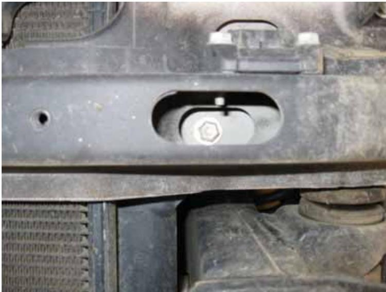
Slide the drop brackets in so the hex bolt goes through the rubber mount and the stud through the original support holes. If you do, you may have interference issues with a nut located on the front bib panel. If you do, you can cut it off or install a stop to prevent your plastic radiator from hitting the nut.
