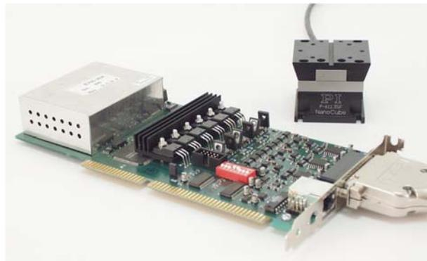
*Fig. 65: E-760 piezo axis controller with NanoCube® in background.*
