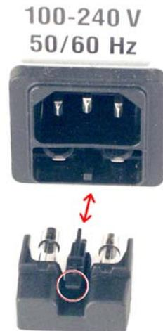
*Fig. 59: Rear panel fuse carrier and fuses*
