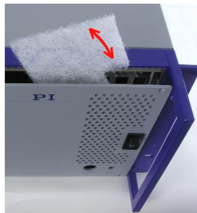
*Fig. 60: Dust filter replacement*
