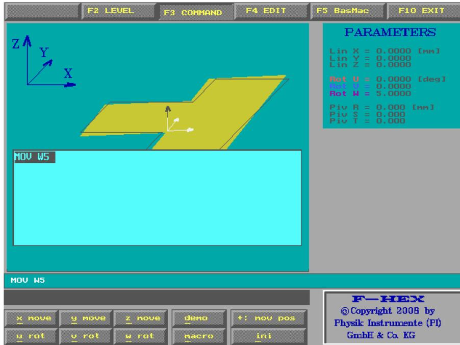
Fig. 19: Command entry, direct on F-206 Hexapod controller; exit with **ESC** to activate other buttons
