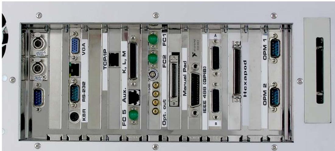
Fig. 71: Controller rear-panel connections and removable media reader. (Note: rear-panel KBD connector inactive on units with built-in keyboard and display).
