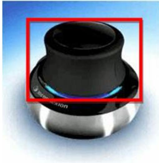
Figure 5: “Joystick” part of the SpaceNavigator.
