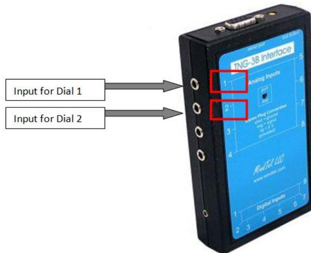
Figure 7: Input ports for Dial 1 and Dial 2 of the TNG-3B Serial Interface
