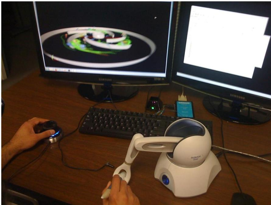
Figure 11: Hold the The Phantom Omni Device stylus like a pen
