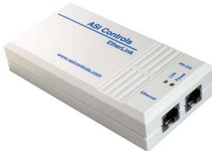
The EtherLink device allows communication with an ASi Control Network over ethernet by means of the ASi OPC Data Server. The EtherLink Device has an Ethernet connection that can be configured with an IP Address. The EtherLink Device has an RS-232 connection that can be configured with a baudrate.
