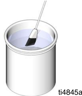
FIG. 15: Use solvent-dipped soft-bristle brush
