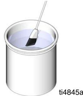
FIG. 14: Use solvent-dipped soft-bristle brush
