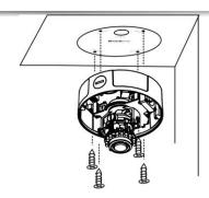
WARNING: Do not mount the camera on any soft material. The camera may fall and be damaged.POE, Power, DIDO, Audio Connection:
