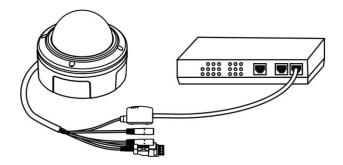
ii. Connect the camera to a non-PoE switch using the PoE Injector.
