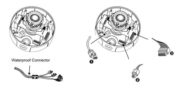
A compliant waterproof connector shall be attached tightly to the conduit hole of the Vandal Dome Network Camera, and all the cables shall run through the connector for the camera to be IP67-compliant.
