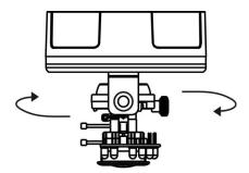
ii. Release the tilt screw on both side of the device to tilt the lens up or down. After completion, tighten the tilt screw.
