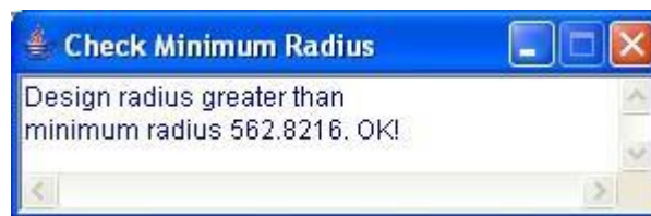
Figure 4(b) Check minimum curve radius
