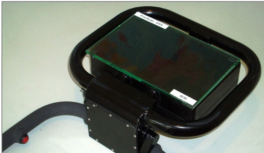
Figure 21 - checking the calibration with the glass plate
