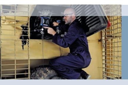
81301001-415 MoVeo VIDEOSCOPE 1.5 m x diameter 4 mm, Set,
