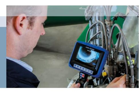
MoVeo functions on both mains and internal batteries, making it suitable for stationary and mobile operation. The MoVeo videoscope can operate for up to 3 hours on the rechargeable lithium-ion battery.
