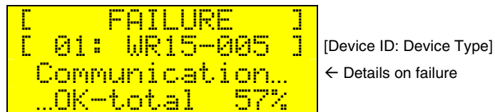
Fig. 4.15: Details on failure
