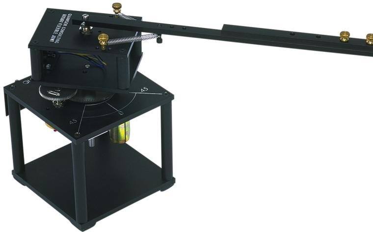
Figure 1.1: SRV02 Rotary Flexible Joint Module
