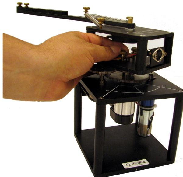
Figure 4.1: Attaching ROTFLEX to the SRV02
