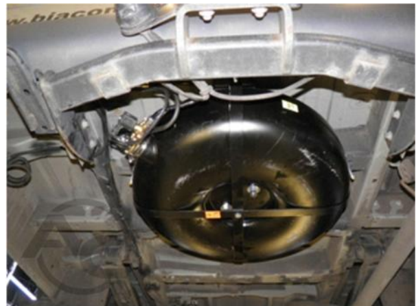
Photo 5. Installation of the gas tank in a minibus
