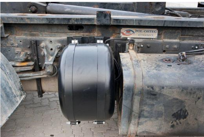
Photo 4. Installation of the gas tank in truck
