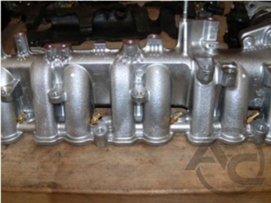
Photo 7. Position of nozzles in the manifold (outside view)
