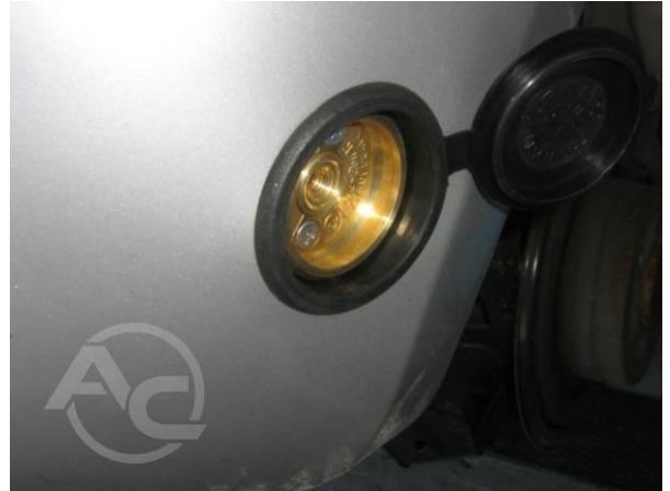
Photo 3. Installation of the filling valve in passenger cars
