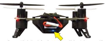
Please disconnect the battery before the memory card is inserted or removed from the camera. When KODO is linked with the controller and the card is installed correctly, there will be a steady blue LED just above the card. A red LED flashing next to the blue LED when the camera is not operating indicates that the card is missing or not installed correctly.
