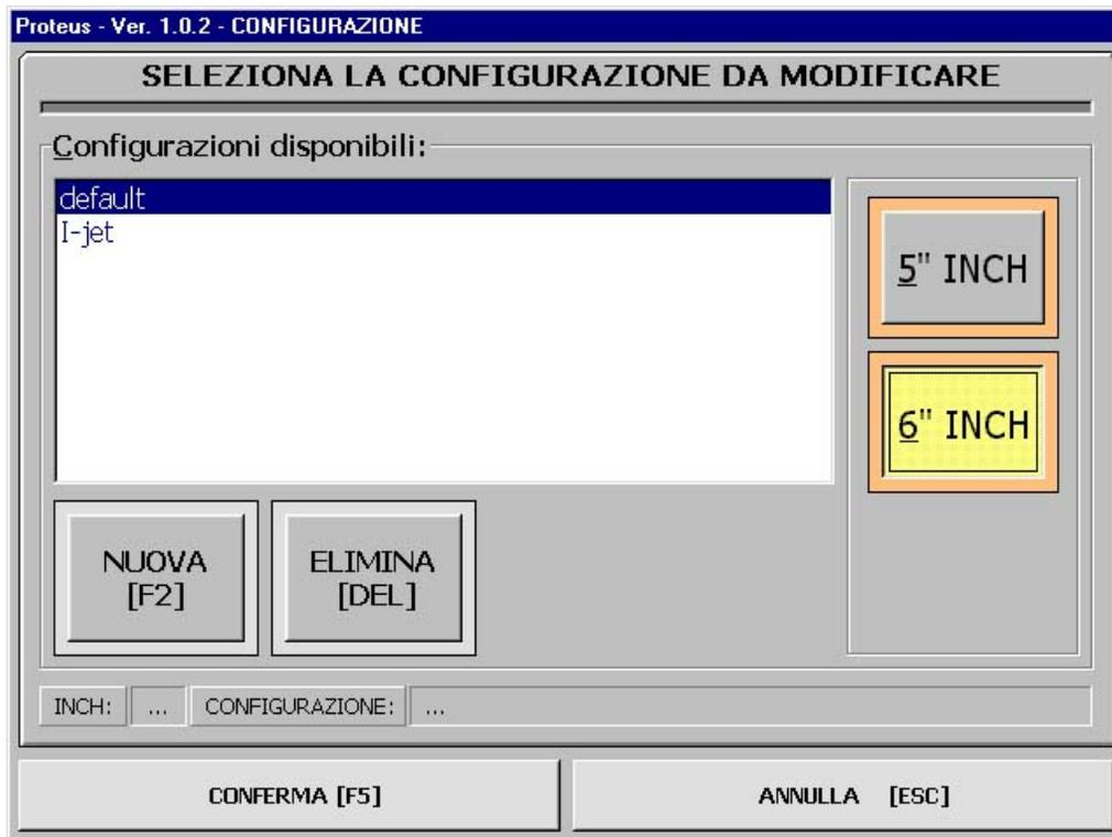
Select before wafer size and then the recipe by clicking its name, then press CONFIRM (F5) to load.
