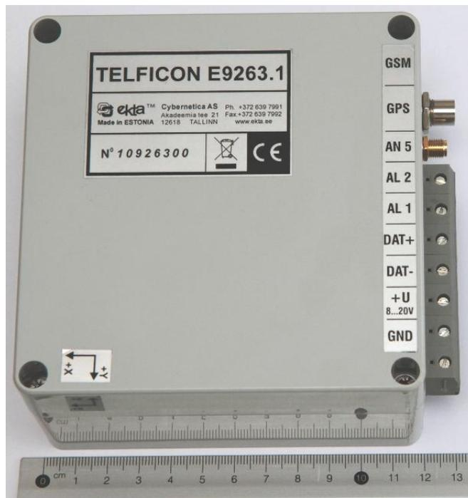
Figure 1. Electronics module of the TelFiCon E9263.1 Set, view from above.
