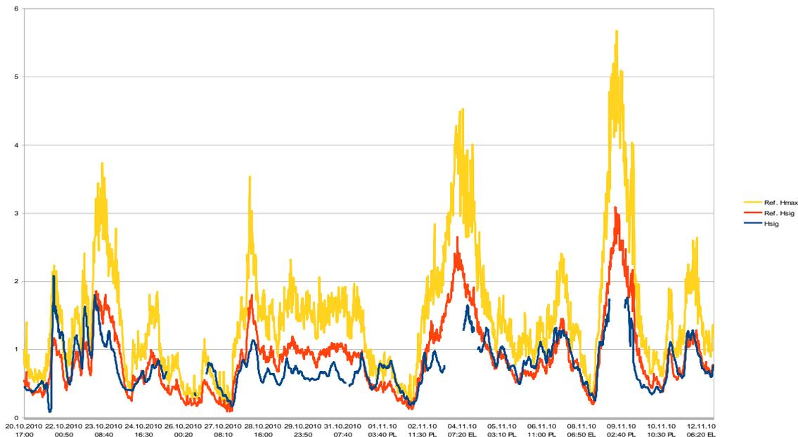
**Figure 19** Significant wave height as measured by acceleration sensor on navigation buoy NM159 (blue) and pressure sensor based probe (red) in Kuradimuna, second measurement period. Yellow line shows maximum wave height recorded by pressure probe.
