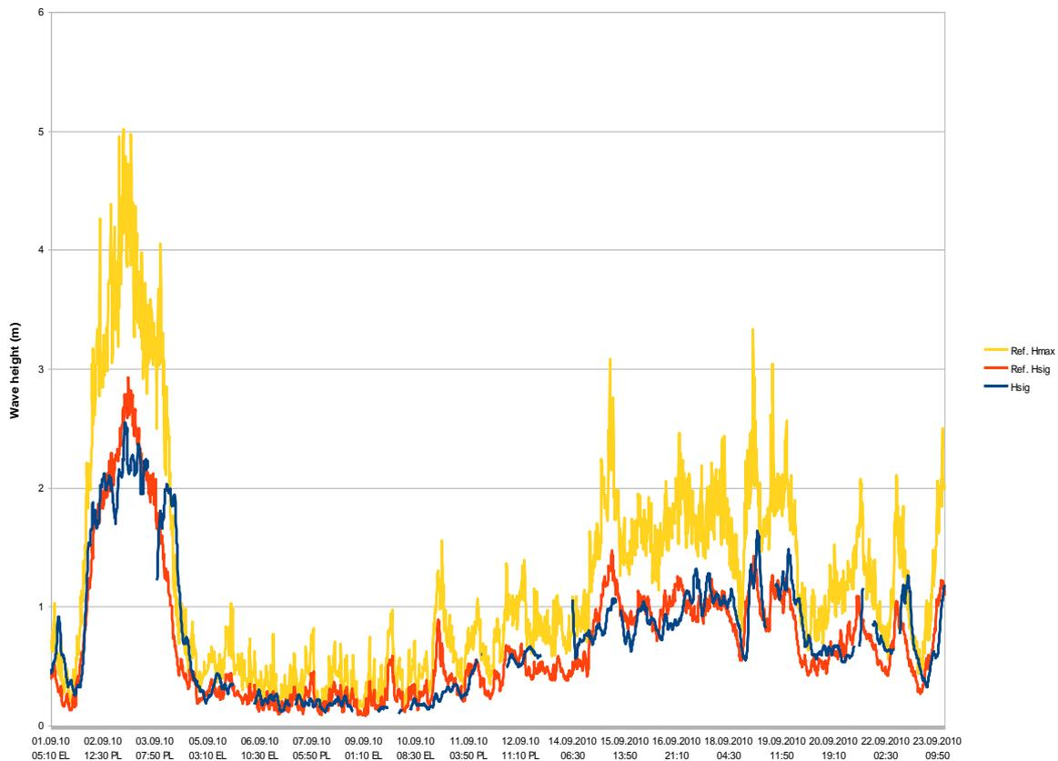
**Figure 15** Significant wave height as measured by acceleration sensor on navigation buoy NM157 (blue) and pressure sensor based probe (red) in Kuradimuna, first measurement period. Yellow line shows maximum wave height recorded by pressure probe.
