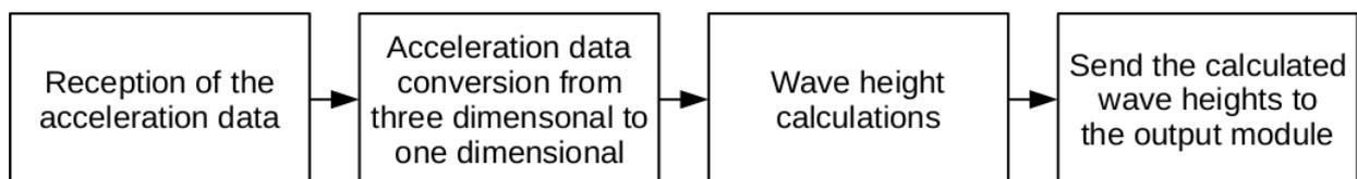
*Figure 3. Flow diagram of WCSC operation*
