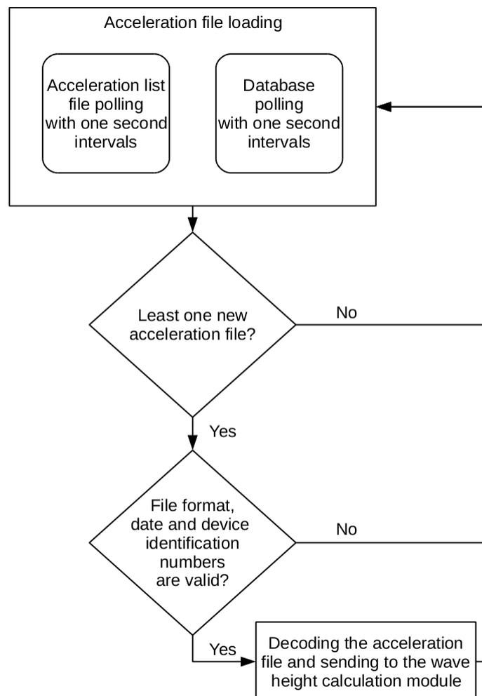
Figure 2. Flow diagram of DRSC operation
