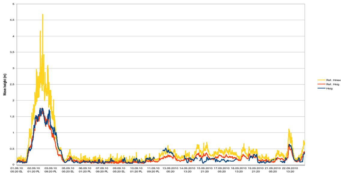
**Figure 13** Significant wave height as measured by acceleration sensor on navigation buoy NM186 (blue) and pressure sensor based probe (red) in Karbimadal, first measurement period. Yellow line shows maximum wave height recorded by pressure probe.
