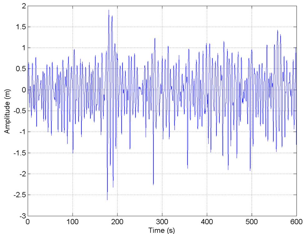
**Figure 6** Snapshot of *in situ* wave package during 10 minute long time sequence, measured with pressure sensor, high variability in wave heights during that short time period could be easily observed from the graph.
