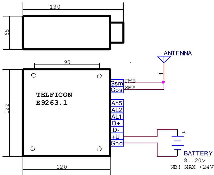
Figure 3. TelFiCon E9263.1 dimensions and connections
