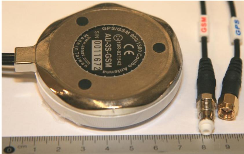
Figure 2. GSM/GPS antenna TecSys AU-3S-GSM with magnetic mount supplied in the E9263 Set
