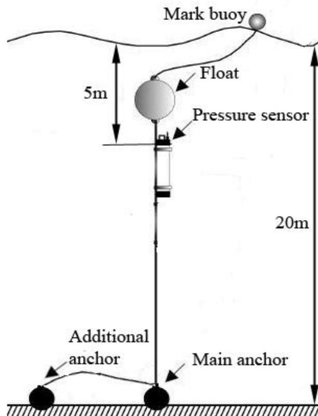
**Figure 8** Scheme of the mooring at the wave measurement stations in Karbimadal and Kuradimuna
