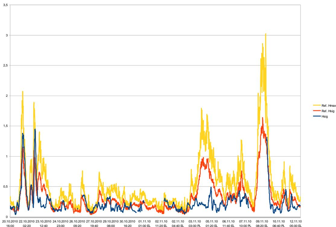
**Figure 20** Significant wave height as measured by acceleration sensor on navigation buoy NM186 (blue) and pressure sensor based probe (red) in Karbimadal, second measurement period. Yellow line shows maximum wave height recorded by pressure probe.
