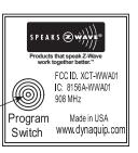
**Inclusion in (adding to) a network:** 1) Set up the inclusion mode at the controller; 2) Press and hold the button for approx. 2 seconds until the controller indicates the unit has been included in the network. Also, a beep will be heard when the inclusion completes. Inclusion and exclusion are always done at normal transmit power mode.
